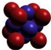
Face-Centered Cubic Structure
